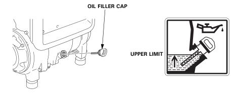
The Oil Alert system will automatically stop the engine before the oil level falls below safe limits. However, to avoid the inconvenience of an unexpected shutdown, check the oil level regularly.
